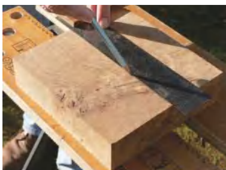
▲ Pic.1 Cut your timber to size, cleaning up sawn edges with a plane or disc sander; on wild grain a belt sander is an easy way to smooth the top. Mark two centrelines...
